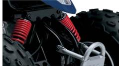
**Independent single A-arm coil spring, oil damped front suspension** delivers a comfortable ride over all types of terrain.
