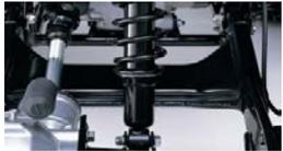
**Swingarm-type rear suspension** features single shock absorber with 5.9 inches of ground clearance for impressive performance over rough trails and terrain.
