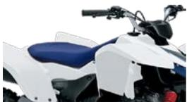
**Strong, high-rigidity steel frame** was designed to be sturdy and compact to withstand any conditions off road or from the rider. The QuadSprt Z90 also features modern styling with full floorboards and a big Quad look, plus white paint and graphics
