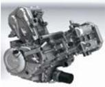
**1037cc, 90 degree V-twin, DOHC, eight-valve, liquid-cooled engine** produces class-leading power with ample torque and horsepower for outstanding performance on or off the road. Dual-spark heads provide improved combustion and reduced emissions. Combined with a 32-bit Engine Control Unit (ECU), state-of-the art Suzuki Dual Throttle Valve (SDTV) fuel injection and a transmission tuned for sporty riding make the V-Strom 650 the choice to make adventure tours more enjoyable.
