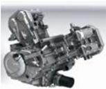
**645cc, 90 degree V-twin, DOHC, eight-valve, liquid-cooled engine** produces class-leading power with ample torque and horsepower for outstanding performance on or off the road. Dual-spark heads provide improved combustion and reduced emissions. Combined with a 32-bit Engine Control Unit (ECU), state-of-the art Suzuki Dual Throttle Valve (SDTV) fuel injection and a transmission tuned for sporty riding make the V-Strom 650 the choice to make adventure tours more enjoyable.
